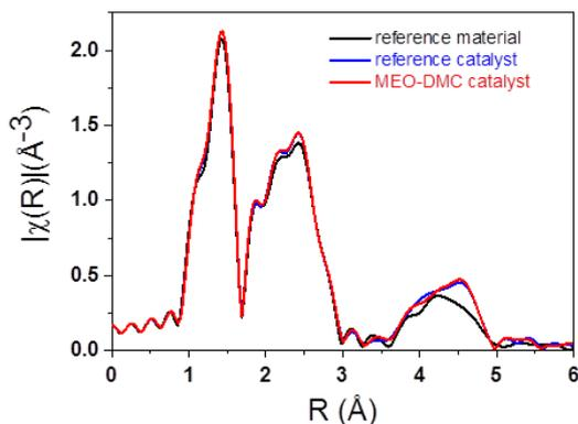
Figure 3. The comparison of FT modules of the experimental Co K-edge spectra for investigated materials.
