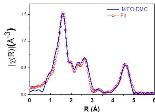
Figure 2. Fit of the EXAFS data to the final model of the local atomic structure around Zn atoms for MEO-DMC catalyst.
