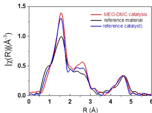
Figure 1. The comparison of FT modules of the experimental Zn K-edge spectra for investigated materials.
