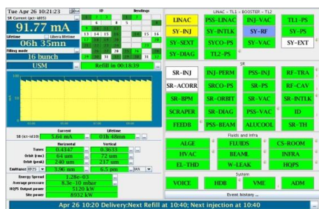
Figure 2. Top-up operation in 16-bunch mode. This snapshot of the control room synopsis screen shows the 20-minute injection periods and a low vertical emittance of 6.5 pm rad.
