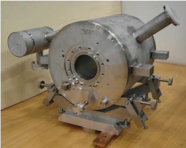
Figure 4. XFEL superconducting magnet.
