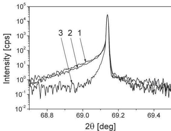
**Figure 1.**  $2\theta/\omega$  X-ray diffraction patterns (004 Si reflection) for Czochralski Si:Mn samples annealed for 1 h at 340°C (1), 600°C (2) and 800°C (3).
