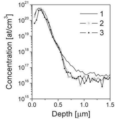
**Figure 3.** SIMS Mn depth profiles for Czochralski Si:Mn: as-implanted sample (1) as well as for samples annealed for 1 h at 600°C (2) and 800°C (3).
