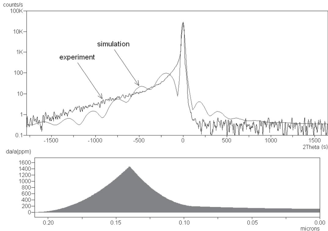
**Figure 5.** Numerical simulation of  $2\theta\omega$  X-ray diffraction pattern (upper) and depth distribution of the Si-matrix strain (lower) for Czochralski Si:Mn sample annealed for 1 h at 340°C.
