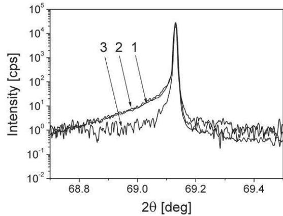
**Figure 2.**  $2\theta/\omega$  X-ray diffraction patterns (004 Si reflection) for Floating-zone Si:Mn samples annealed for 1 h at 340°C (1), 600°C (2) and 800°C (3).
