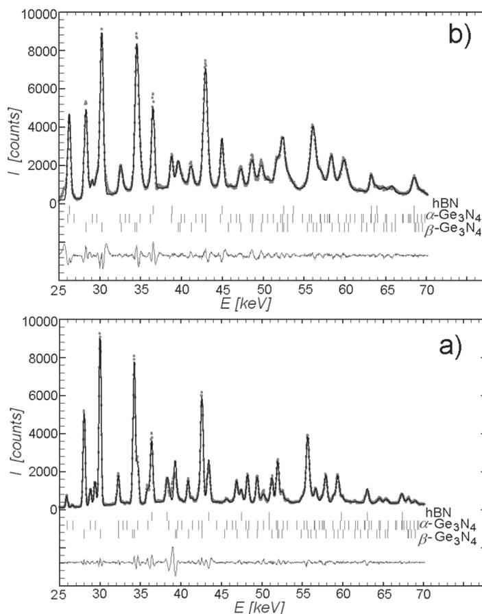
Figure 1. Examples of spectra collected at the ambient (a) and 5.0 GPa (b) pressures, fitted using the Le Bail method.
