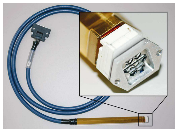
Figure 1. Photograph of a complete detector module, the inset shows the head of the detector with the AlN housing (white) and a Zr mask in front of the SDD chip.
