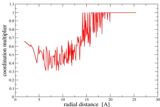
Figure 3. Ratio of Radial Distribution Function (RDF) of model 2 to that of model 1.
