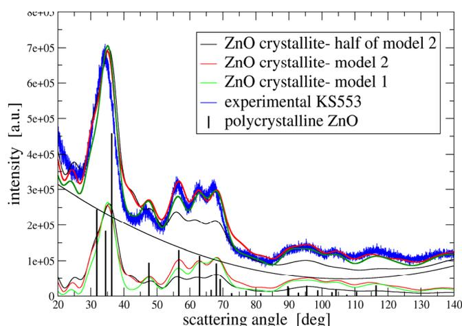
Figure 2. XRD pattern of the nanocrystalline ZnO sample compared to diffractograms of models
