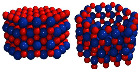
Half of the model 1: a regular fragment of ZnO lattice. Zn- blue, O- red. Half of the model 2: a crystallite with empty interior.
