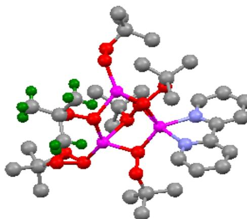
Figure 1. Unit cell view of the crystal serving as a precursor to the studied nanocrystalline sample. Atom colors: Zn atoms- magenta, O in red, C in grey, N in light blue and part of H atoms in green.
