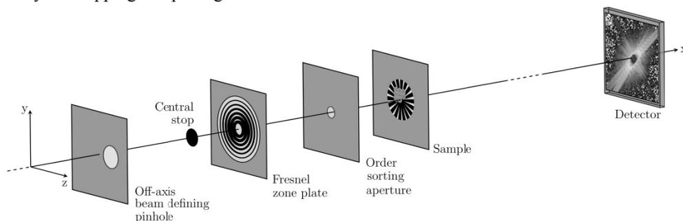
Figure 1. Schematic of the ptychography experiment using an off-axis illuminated zone plate.
